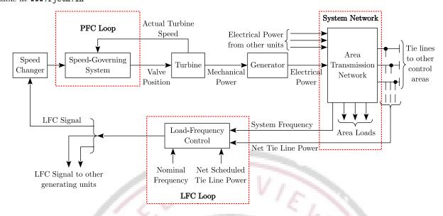
Figure 1: The Basic Schematic of Load-Frequency Control in Power System
