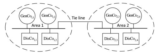
Figure 4: Single Line of a 2-Area Deregulated System
